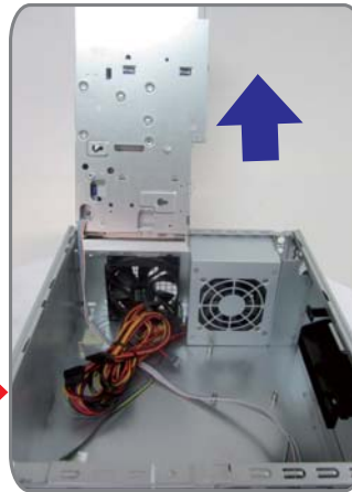
Remove the screw and rotate the bracket (cradle) at the position with angle 100 degree.
