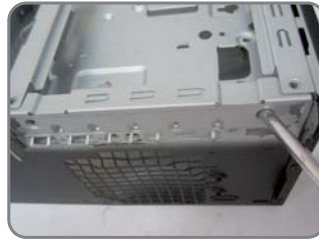
Disassemble the half-punched metal cover to take it out
