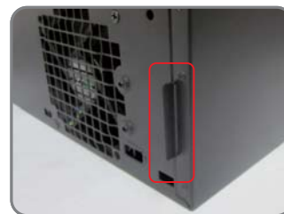
Remove this half-punched metal bracket
