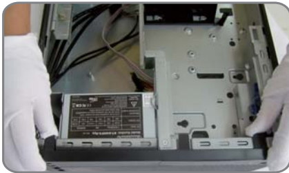
Remove the front panel
