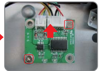
Fit the PCB with 2pcs M3 screw, the cable should be at the top side.
