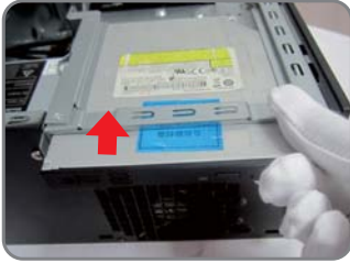
Slides off the side cover upwardly
