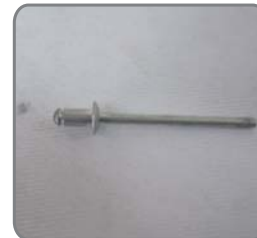
If PC shot down and the lock has been closed, the top cover can't be removed. User could use this nail (shown as picture) to push out the lock pin of solenoid lock inside PC, then top cover could be removed.
