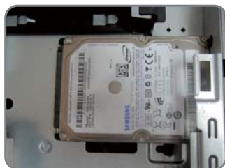
open the cradle and put the 2.5HDD at this place (note: please pay attention the HDD might fall down).
