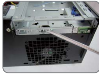
Remove the half-punched metal cover
