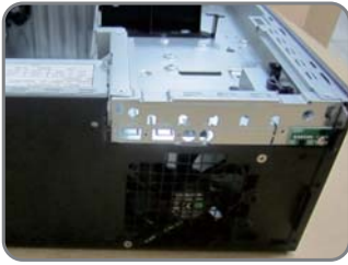
Slides off the side cover upwardly
