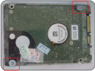
fitting 2pcs "E" screw on 2.5"HDD
