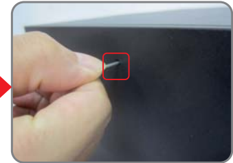
If PC shot down and the lock has been closed, the top cover can't be removed. User could use this nail (shown as picture) to push out the lock pin of solenoid lock inside PC, then top cover could be removed.
