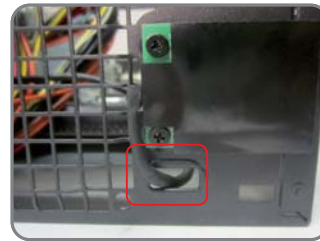
let the cable go through this hole as shown on picture.
