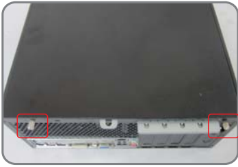
Disassembly of 2pcs thumb screw
