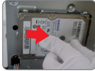
fit the HDD on cradle , push and move it as the RED arrow direction
