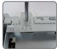
Remove the screw and rotate the bracket (cradle) at the position with angle 100 degree.
